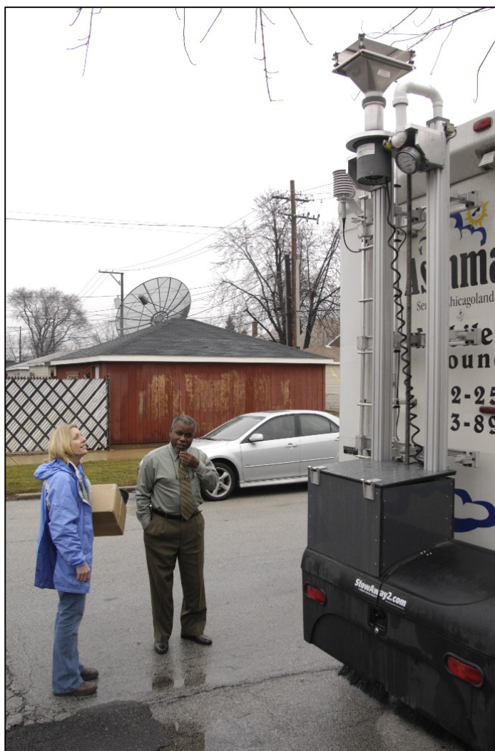
Figure 2-3: Implementation of the Hi-Vol samplers onto the backs of the asthma vans (photo courtesy of Timothy Schoon, University of Iowa)
